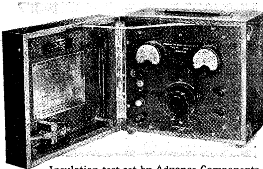
Insulation test set by Advance Components.
